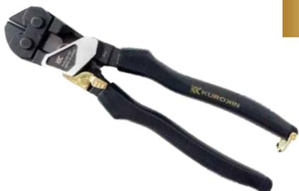
This tool allows you to cut steel wire up to 4mm with one hand. Easily cut the 4mm wire used when setting up scaffolding. The design enables the entire process taking the tool from the waist bag, releasing the lock, and cutting the wire to be completed with one hand, improving efficiency in narrow and unstable environments.
