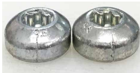
Figure 1: “Closed” Head Cracks
