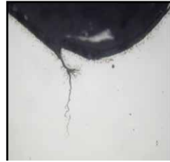
Figure 8: Example of Thread Lap at Thread Root
