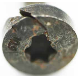
Figure 5: Example of a Shear Burst
