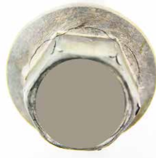
Figure 7: Example of Folds in Hex Flange Head
