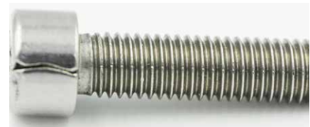
Figure 3: Example of Head Crack Due to Wire Seam (Note seam running through the threads.)
