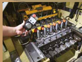
Dial Control Style Slow Jog System 手搖輪慢寸動功能
