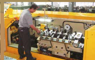
Transfer Housing Lift & Turn System 夾仔台旋出機構
