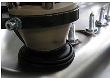
Graphic 2. The best orientation to weld studs shows gas cover and secondary shield boot.
