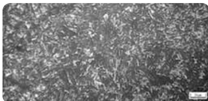
▼ Figure 9. Oil-quenched M16×120 Bolt, Grade 6 (ML40Cr×500)
