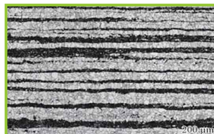
▲ Fig. 1 Ferrite/Pearlitic Structure
