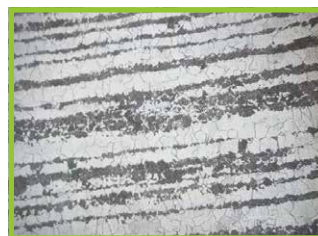
▼ Fig. 2 45 Steel Ferrite/Pearlitic with Banded Distribution
