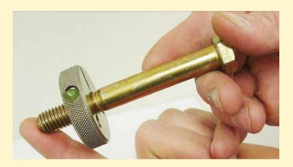
NoGo or Not Go thread ring gages have some not so straight forward rules. You would think that since the name of the gage is NoGo, that it should not even start to go onto the bolt threads. For practical reasons, this is not the case. Also, not all standards actually agree on how far the NoGo thread ring should be allowed to go onto a screw or bolt thread.
