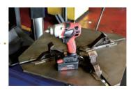
Business Development Manager Michael Gater said "There is an issue with garages over-tightening wheel nuts and studs. This can be just as bad as under-tightening as it can have an impact on the integrity of the thread potentially making the wheel become loose. Torque Master gives peace of mind that nuts will never be tightened to more than 70Nm whilst having the advantage of being able to remove wheels very quickly."
