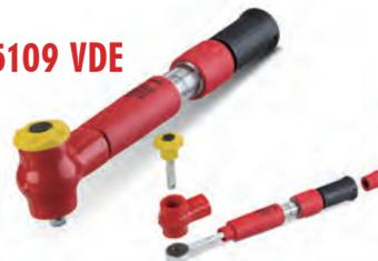
The torque wrenches have been developed for working on live components. In contrast to conventional VDE torque wrenches, which cannot be disassembled and reassembled due to their sheathing, the 5108 VDE and 5109 VDE can be readjusted and recalibrated. The interchangeable square drive enables both right and left tightening. The achievement of the set torque value is signalled palpably with a close-gap release and audibly with a “click” sound.
