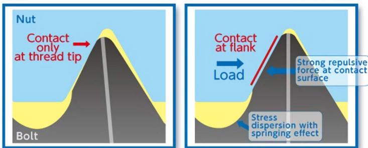
《Before closing》 Thread elastic deformation 《After closing》
