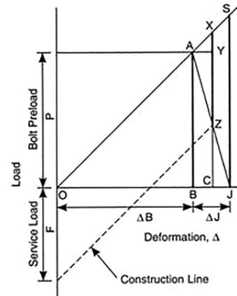
determining what type and size of bolt to use in the joint. The stiffness ratio can also help determine preloads, loss due to embedment and bolt failure.
