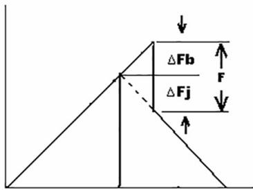
Figure 3. Softer or More Springy Fastener in a Stiffer Joint
