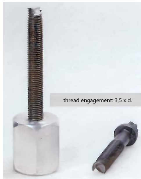
Figure 2. Desired bolt 2-piece failure at 3.5 x diameter of thread engagement.
