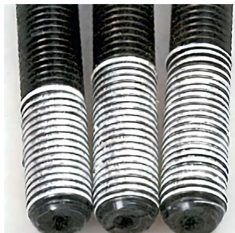
Figure 3. Aluminum internal thread strippage at 2 x dia., 2.5 x dia., 2.75 x dia.
