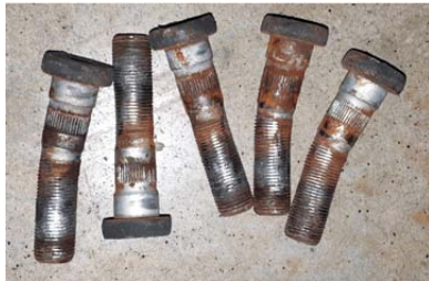
Fig. 7. Deformation of automotive screws
