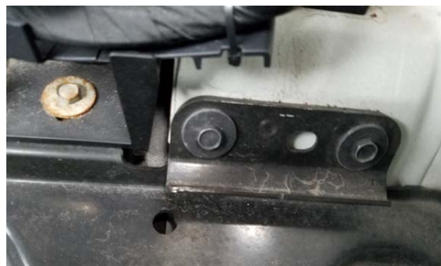
Figure 2: Example of Property Class 8.8 Fastener on Underhood Bracket
