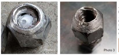
To be sure the wheel is tight, many mechanics will continue to impact the wheel nuts into the wheel boss. Sometimes, as illustrated by the wheel nuts in **Photos 2** and 3. The conical seat of the wheel boss area will also be damaged. These wheel studs may fail long before the wheel becomes detached, yet the empty wheel hole and missing lug nut will likely go unnoticed by the driver until it is too late.
