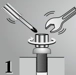
1 Tighten with spanner or cross-recess driver.
