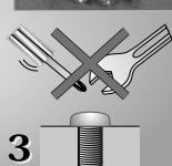
3 After the hexagon head move off, removal is very difficult with the general tool, it's possible to prevention of mischief and theft.
