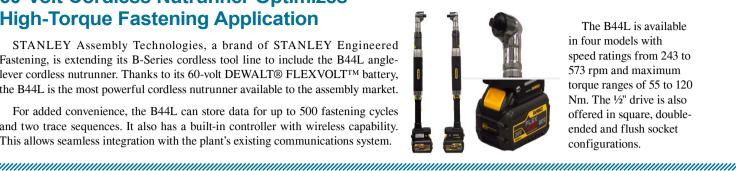
The B44L is available in four models with speed ratings from 243 to 573 rpm and maximum torque ranges of 55 to 120 Nm. The 1/2" drive is also offered in square, doubleended and flush socket configurations.
