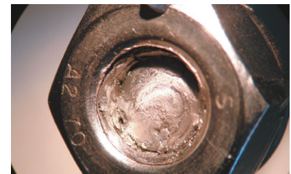
Fig. 8. Cold-weld on the nut A2
