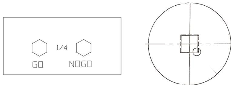
Square driver bits also need to be inspected for the same reasons a Hex bit requires inspection. A bad square driver bit can round out the screw recess resulting in an ineffective drive.
