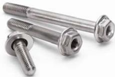
Nevada-based fastener supplier Click Bond is launching its new LoMas screw at this year's Farnborough Airshow. The product is an A286-grade stainless steel screw that is up to 50 percent lighter than alternatives and 17 percent lighter than titanium counterparts. LoMas Screw will initially be available in 10 to 32 thread in 15 lengths from 0.250 to 2.00
