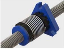
Custom mounting configurations are also available. The design has a shortened nut length to reduce the OAL or increase stroke length for a given lead screw. Modifications can be made as required and this low torque/high axial stiffness design includes a unique machined version for applications that require a smaller nut size due to space limitations.
