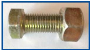
**Zinc** This is a metal that provides a sacrificial barrier between the substrate (bare metal part) and atmospheric corrosion. In other words, it will corrode first, thereby protecting the steel part. It is applied to fasteners in several ways; hot dip, mechanical deposition, electroplated or by chemical conversion. When corrosion begins, it will produce a white corrosion product.
