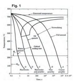
special alloys, such as; A354 BD and SAE Grade 8 cap screws, as well as A449 cap screws 1/4" through 3/4" diameters. The SAE J429 permits water quench on grades 5 and 5.2. Larger diameter A449 fasteners may be quenched in water. The choice of the quenching liquid is determined by the amount of heat which must be dissipated, a function of the cap screw's cross-sectional area of diameter, and the steel to be quenched.
