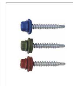
Hex Washer Head Self Drilling Screw With EPDM Washer, #2, Zinc Plated/Painted
